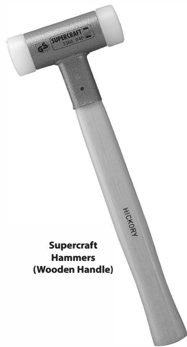
No-Rebound Hammers are filled with special steel pellets that transfer momentum to the impact point.
